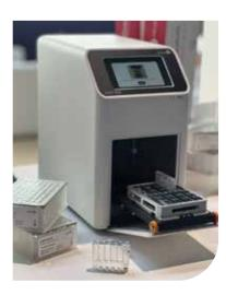
Genes2Me Rapi-X16 nucleic acid extraction system features high sensitivity with precise mechanical movement. The system ensures homogenous suspension and distribution of magnetic beads, leading to higher DNA/ RNA yields.
